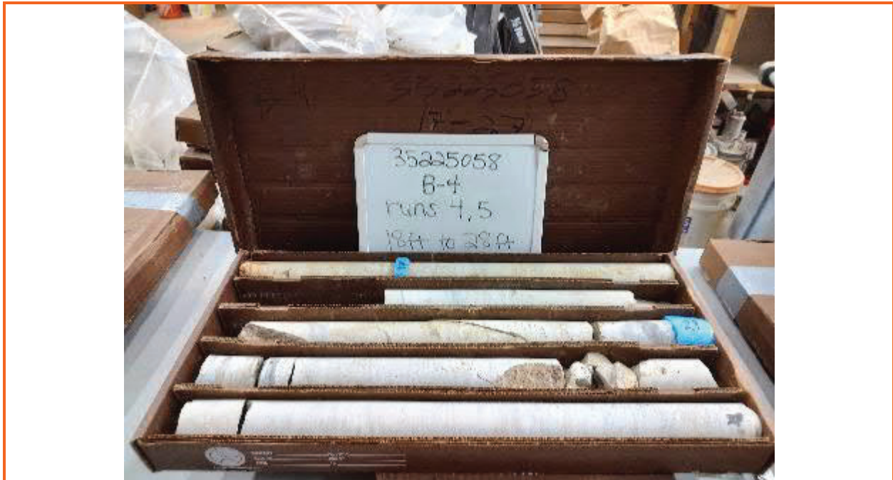
Boring B-4 core run 4 and 5
