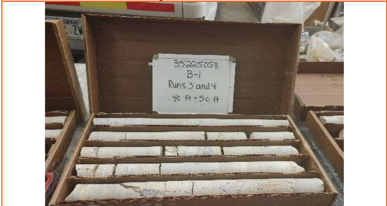
Boring B-1 core run 3 and 4
