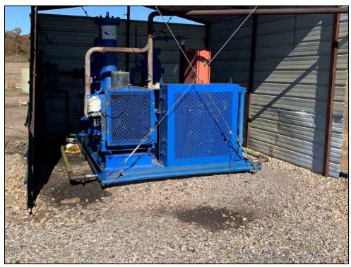
**Photo 9:** Oil staining on gravel around diesel-powered compressor at Stephens Production – Newton, Don #1 well head.
