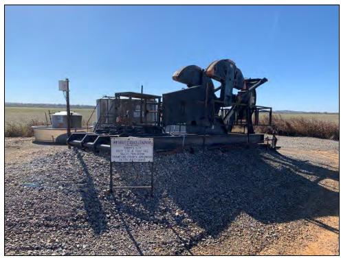
Photo 19: View north of Merit Energy Company, LLC. – Tibbitts #5-11 well head (Exhibit 2, Map ID #8) located west of Thornhill Street south of Kibler. Well head on right side of pump jack.
