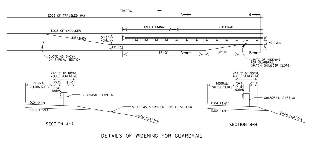
NOTE: NORMAL SECTION TO BE WIDENED APPROX. 5'-6" EACH SIDE TO SUPPORT GUARDRAIL.
