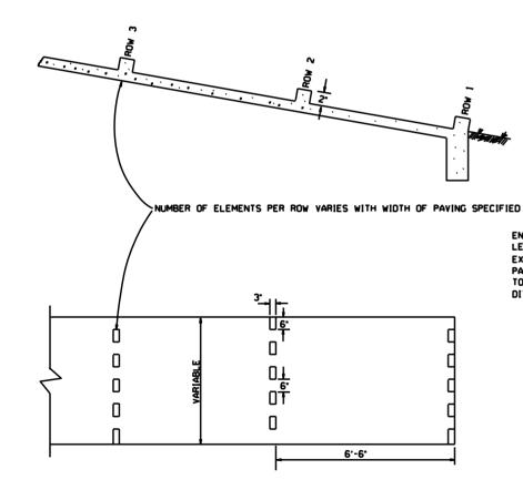
ENERGY DISSIPATORS TO BE USED FOR THE ENTIRE LENGTH OF DITCH WHEN SLOPE OF DITCH PAYING EXCEEDS 7%. THE DISSIPATORS WILL NOT BE PAID FOR DIRECTLY, BUT SHALL BE CONSIDERED TO BE INCLUDED IN THE PRICE BID FOR CONCRETE DITCH PAYING.
