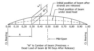
"X" Is Dead Load Deflection of Slab + Diaphragms + Composite Dead Load
