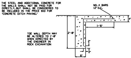
TOE WALL DETAIL FOR CONCRETE DITCH PAVING
