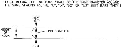
NOTE: DIMENSIONS OF BARS ARE MEASURED OUT TO OUT OF BARS.
