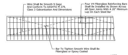
NOTE: All panels shall be braced as required to prevent racking. All parapet joints shall be sawed as soon as practical to a minimum width of ¼". To control cracking before sawing, all joints must be grooved before the concrete is set. Sawing of the joints must be controlled so it will follow the grooved joint.
