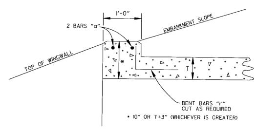
NOTE: FOR ALL SKEWED R.C. BOX CULVERTS THE LENGTH "K" OF THE MODIFIED HEADWALL SHALL BE EQUAL TO THE ROADWAY LENGTH "RL". THE ENDS OF THE HEADWALL SHALL BE CONSTRUCTED PARALLEL TO THE SKEW ANGLE OF THE BOX CULVERT.
