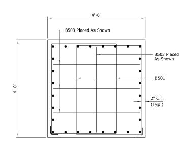
VIEW Z-Z (Typ. both ends of cap) Scale: 1" = 1'-0"
