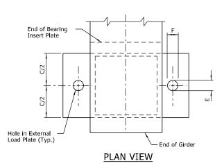
Prior to erection of the girders, the Contractor shall verify the orientation of the bearings with respect to T<sub>a</sub> and T<sub>b</sub>.
