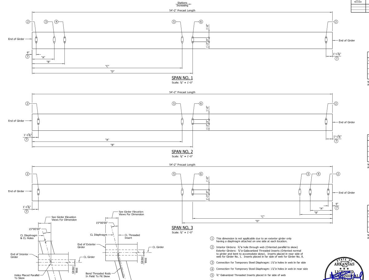
(6) ¾" Galvanized Threaded Inserts placed in near side of web
