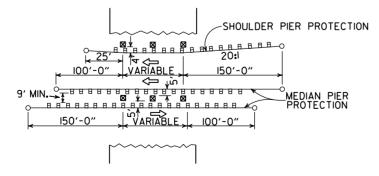
METHOD OF INSTALLATION OF GUARDRAIL AT FIXED OBSTACLE
