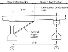
Stage 2 external supports at Girder 5 shall remain in place until after completion of the Stage 3 deck pour. See Subsection 802.15 for additional information regarding the removal of the support system.
