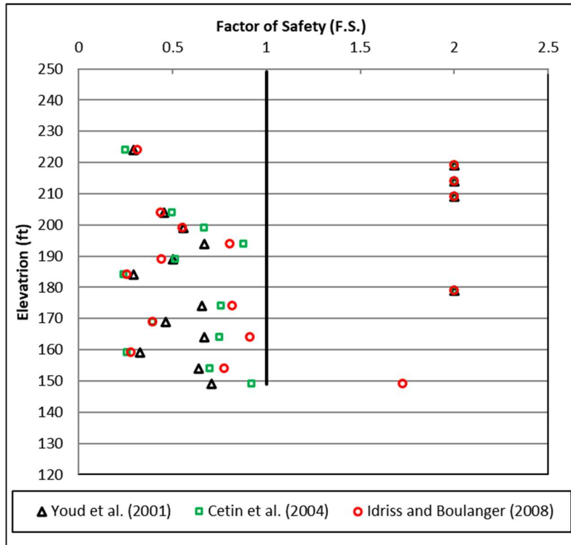
Figure 12 - Liquefaction Triggering FS Values for S1-3 (Top of Boring at EL 249 ft)
