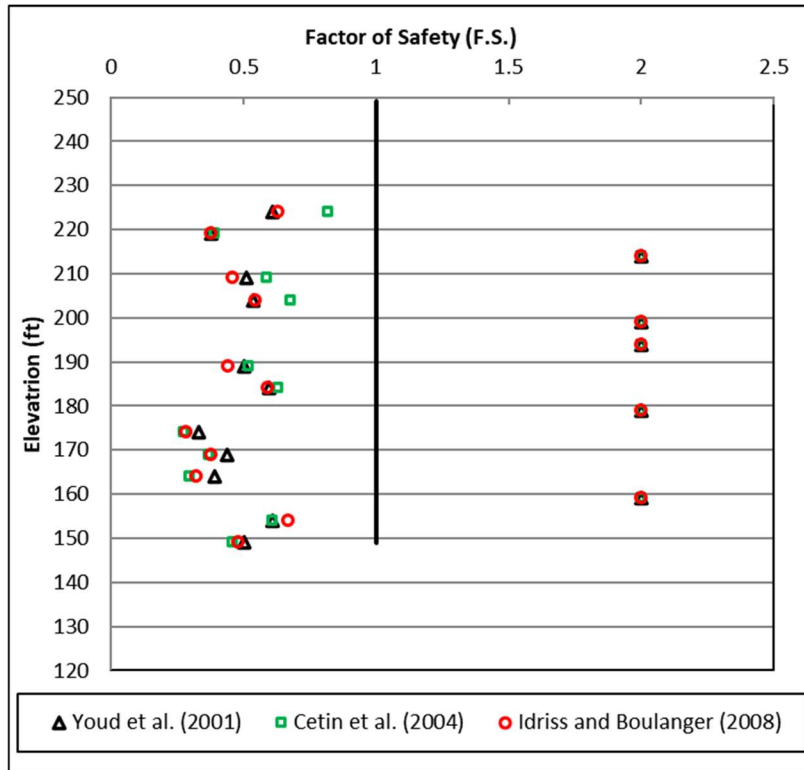
Figure 10 - Liquefaction Triggering FS Values for S1-1 (Top of Boring at EL 249 ft)
