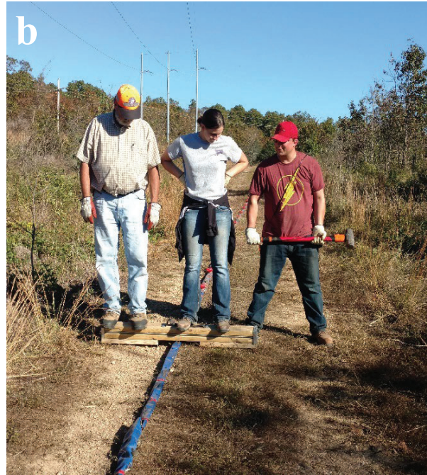
Figure 2.4- MASW testing using Love type surface waves. a) horizontal geophones leveled and oriented, b) wooden shear beam.
