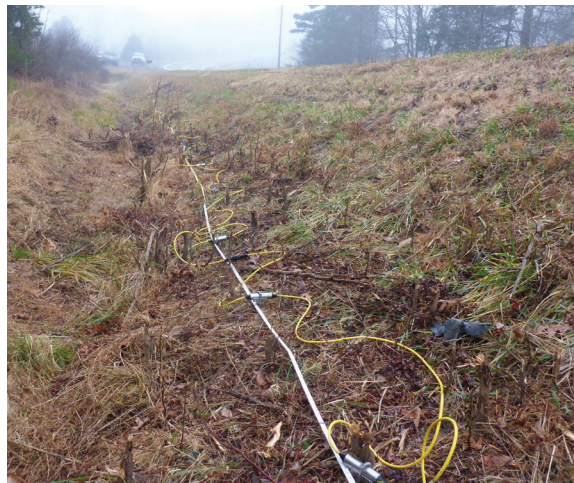
Figure 2.7- ERT survey conducted at the Sand Gap site on the Eastside of Highway 7.
